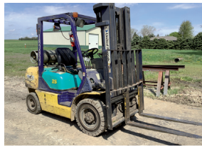
Komatsu Model FG25T-12 Forklift, Nissan Gas/LP Engine, Hyd Fore/Aft, Side Shift, Left Hand Reverser
