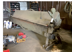
Hyd Metal Break Hyd Pump w/ Reservoir, 3 phase
