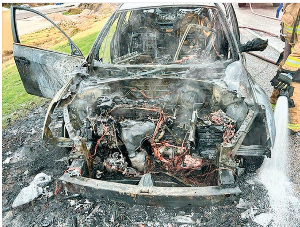
A closeup of the Nissan's burnt-out hood where the fire likely began.
