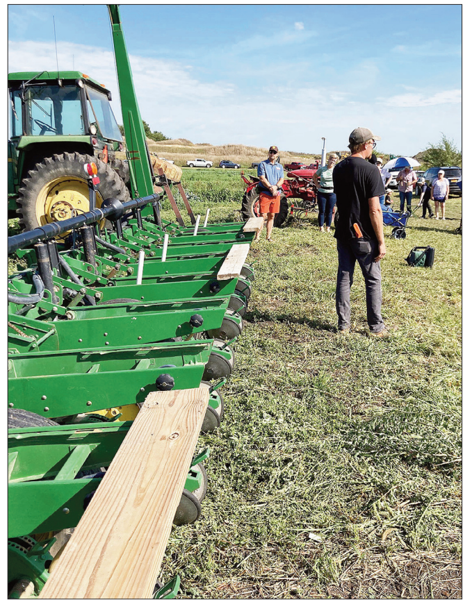
Wooden benches are attached to the planter so helpers can ride along and assist in the seeding process.
