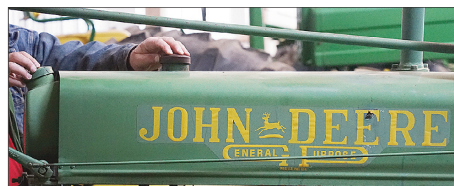
The older John Deere tractors ran on kerosene AND gasoline. Gas was more expensive and more explosive, but was needed to start the engine (an issue of temperature). Argotsinger's right hand is on the cap for the one-gallon gas tank, and his left hand is on the cap for the bigger kerosene tank.
