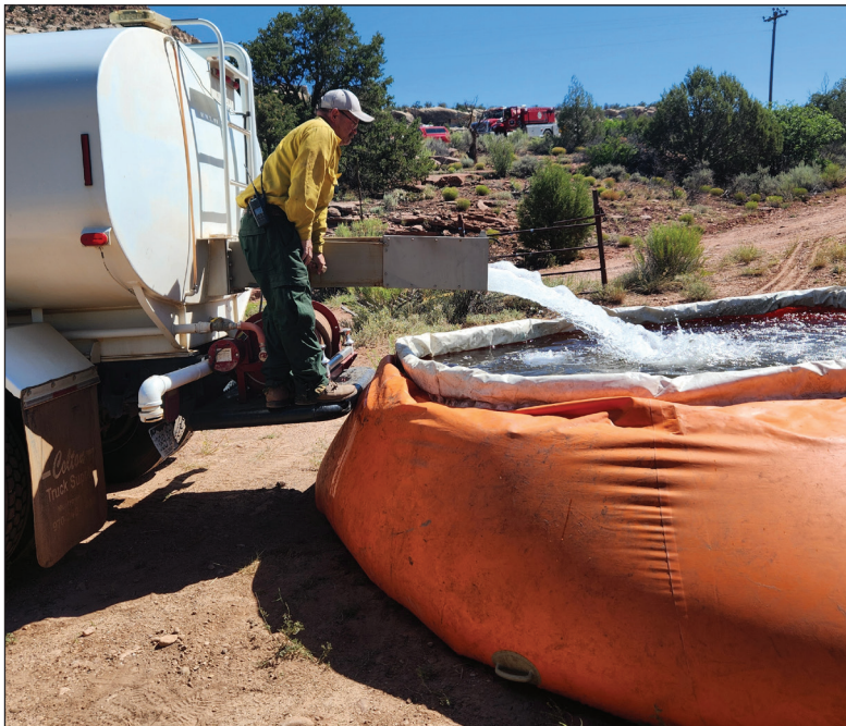
This image shows the filling of the “pumpkin.” (Photo by Ken Jenks)
