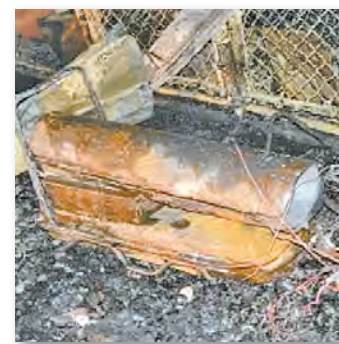
The cause of the blaze which destroyed the No Dogs Left Behind shelter last year -- a salamander heater.
