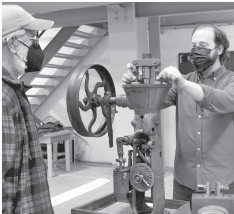
Doug Welch checks out the speed governor of hydro turbines used by Northern Power and Light, demonstrated by owner Emmett Smith at the 2022 Green Living Fair.
