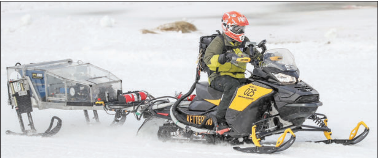
TESTING — Emissions testing was just one of several tests that were conducted on snowmobiles during the SAE Clean Snowmobile Challenge held at the World Championship Derby Complex (WCDC) last week. —Contributed Photo
