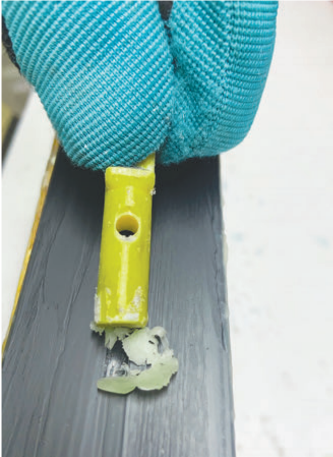
Use a groove pin as the inexpensive but effective tool to prep your ski bases' groove.
