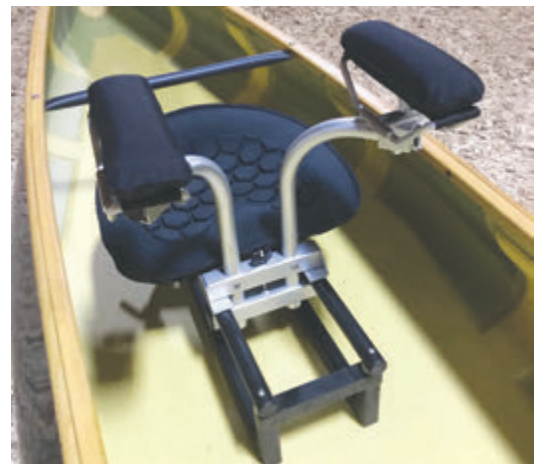
CVCA Solo Pedestal Yoke. A yoke solution for serious portages.
