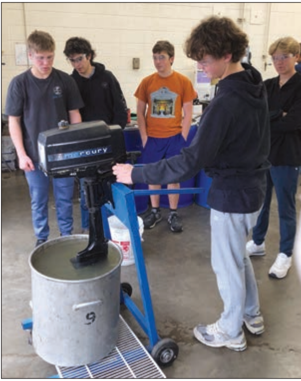
After some carburetor and recoil work in the Tomahawk High School (THS) Small Engines class, this outboard was ready for the test.
