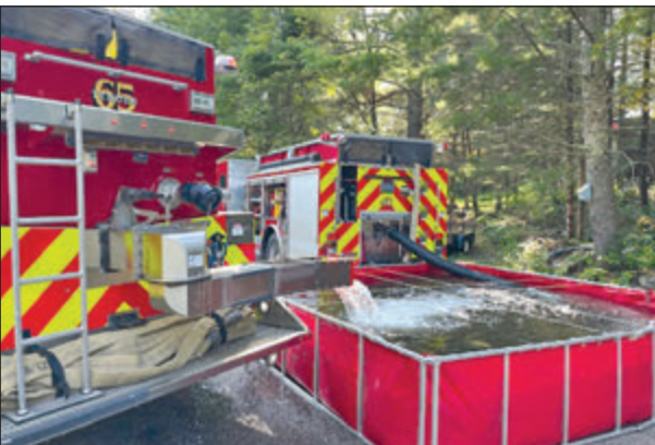
Tender 65 fills a portable water supply tank while another unit draws from the tank to fight the fire.
