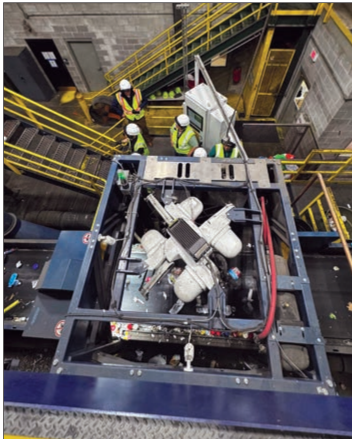
The Tri-County Material Recovery Facility uses several AI robots in the sorting process. Mark Walter photo
