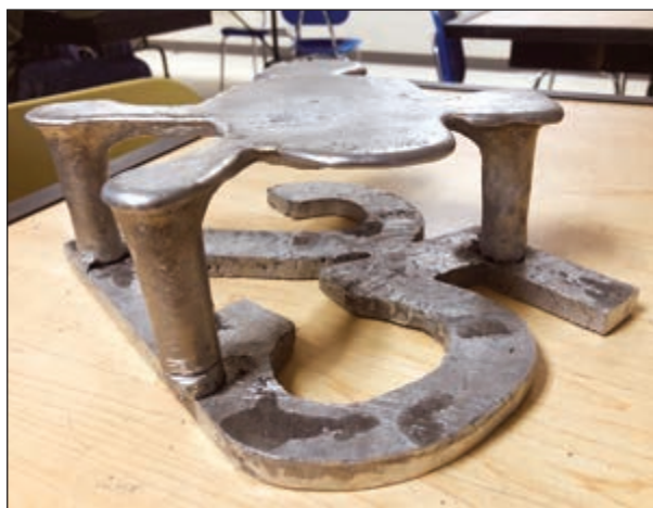
Kashton and Blake poured this project the following day, after which, they cut off the sprues and polished the metal to the desired finish.
