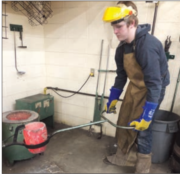
THS Technical Metals students Kashton and Blake pour aluminum into a sand mold.
