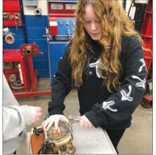
Small Engine students recently began the process of tearing down their engines before cleaning, inspecting, measuring and reassembling their projects. Photos courtesy of Brian Schiltz
