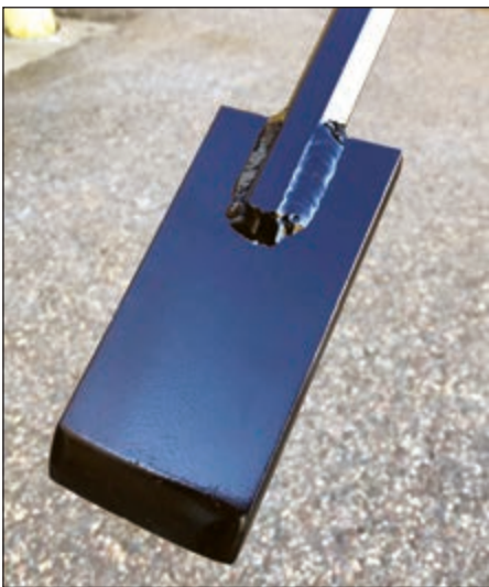
Tomahawk High School (THS) Technical metals students are working on their SMAW welding skills with 7018 electrodes. Makayla presents one of her welds after spending time dialing in her welder.
