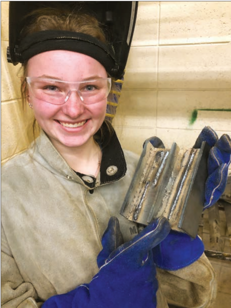
Tomahawk High School (THS) Technical metals students are working on their SMAW welding skills with 7018 electrodes. Makayla presents one of her welds after spending time dialing in her welder.
