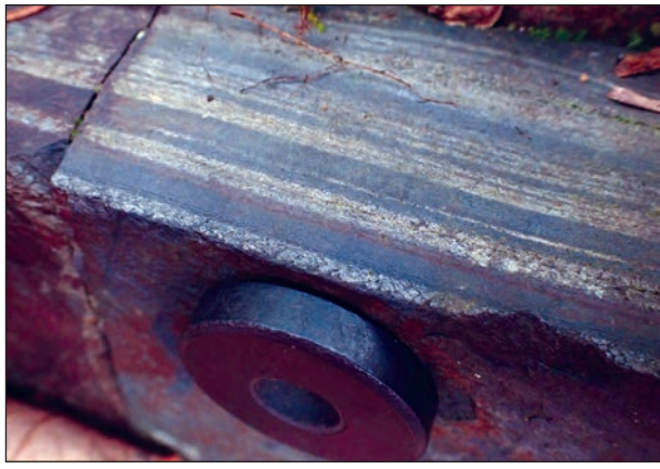
Banded iron formation is made up of layers of different minerals, mostly various combinations of iron, silica and oxygen. Some of the layers are made of magnetite, and so a magnet sticks to the rock outcrop.
