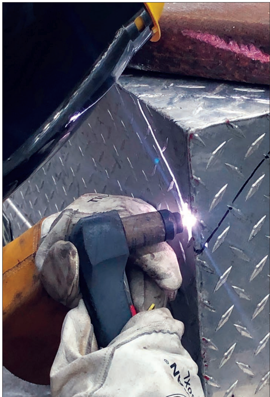
To cut the corners of the aluminum box, Trevor and Blake use a handheld plasma cutter. They will then invert the corners and TIG weld them in place, allowing more room for the box to fit.
