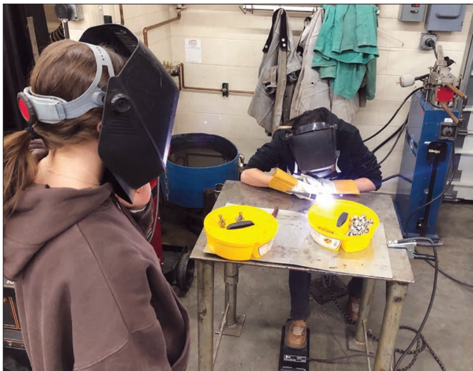
Maddie watches Sophie TIG weld stainless nuts and washers together, creating a festive holiday snowman.
