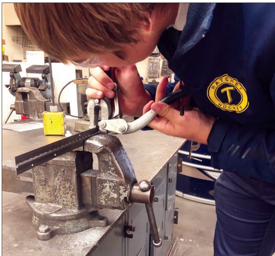
Because Trevor decided to use galvanized steel for his toolbox, he will also use rivets to hold the hinge to the lid and base. He uses a Roper Whitney punch to create the holes in the hinge where the rivets will be installed.
