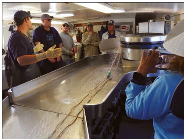
The invention of net lifters (upper right) enabled fishing tugs to become enclosed, which makes for a safer and more comfortable job during the winter. DNR Fisheries Biologist Dray Carl (far left) explains this to participants on a Museum-organized field trip.
