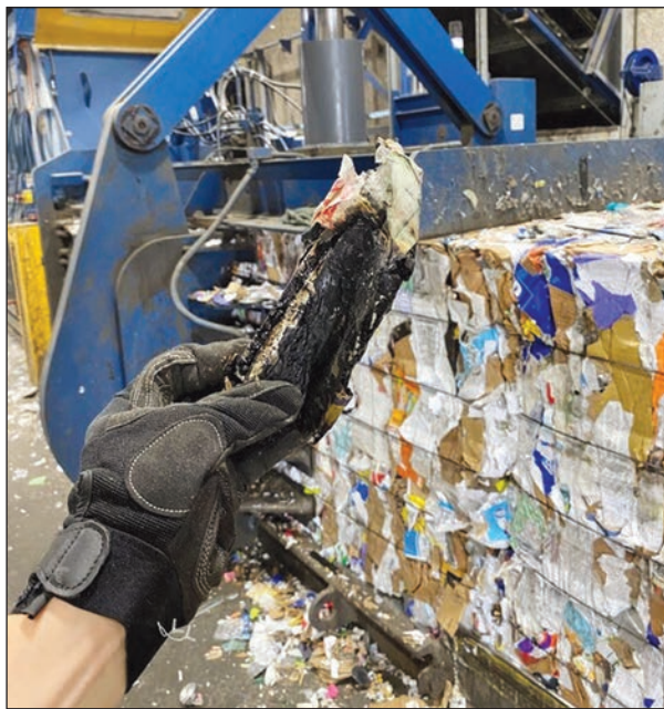
A punctured or bent lithium-ion battery can produce enough heat to melt or ignite materials near the battery, even if the battery itself does not ignite.
