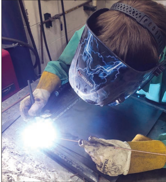
Pictured is the progress Hudson and Brett are making on the sauna stove they have been working on. Hudson is cleaning up some welds on the stove itself, while Brett is TIG welding the door assembly.
