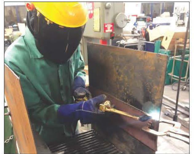
In Metals Fabrication, Brett and Hudson make relief cuts in their wood-fired sauna heater for easier manipulation of the metal. Here they are using pieces of metal as a straight edge while the oxyacetylene torch cuts through the metal.
