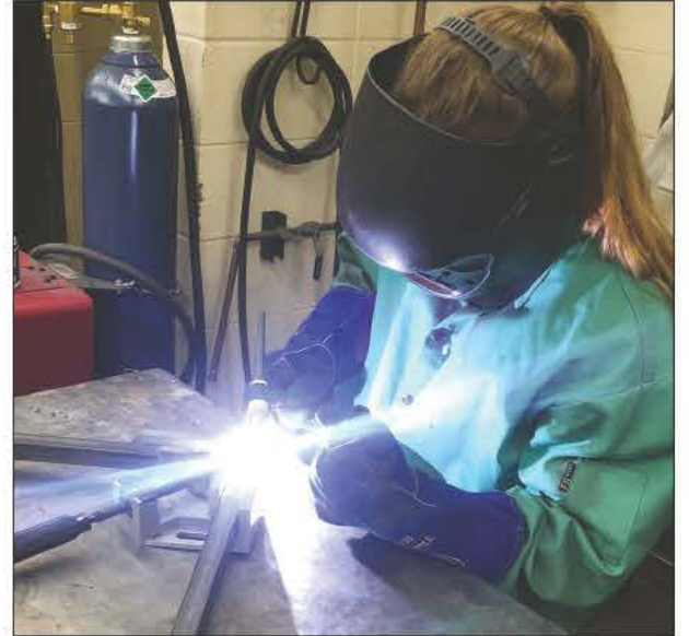
After cleaning and preparing her metal, Mariah begins to tack weld pieces of her infinity table project to ensure proper fit up. She is using the gas tungsten arc welding (GTAW or TIG) welding process in her Metals Fabrication class.
