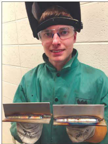
THS Metals Fabrication students recently worked in the shop with a fabricated exhaust tip, figuring speeds and feeds for the lathe and displaying fillet T tig welds on stainless steel.
