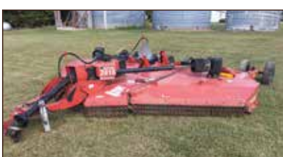
2013 Bush Hog 2815 rotary cutter, front and rear safety chains, laminated wheels, wing fold, 540 PTO
