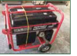
Gentron 10,000 watt generator
