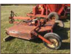
AC pull type 6' cutter, 540 PTO
