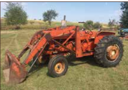
AC D17 Series IV gas tractor, 3 pt., 2 hyd. outlets, 540 PTO, rear weights, 16.9-28 tires, reads 6709 hours, sells with AC 500 hyd. loader, material bucket, runs good.
