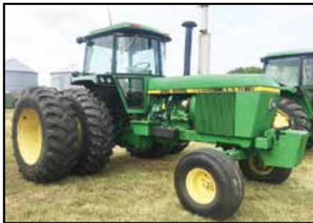
1978 JD 4640 Cab Tractor, 7.6L Cyl Diesel, 16/6 Quad - Range, 2 Hyd. Remotes, 1000 PTO, 10 Front Weights, Sanden AC Compressor Update, 20.8-38 Tires and Duals, Reads 7335 Hours (Approx. 3300 Hours on Overhaul) S# 4640H003500R
