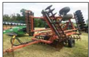
Int 496 24ft Wingfold Tandem Disk, 9in Spacings, 19 1/2 in Front Blades, 20 1/4 in Back Blades, S# 047000U042068
