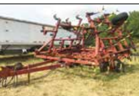
Case-IH 4600 Vibra Shank 28 ft Field Cultivator, Walking Tandems, Rear Hitch, Poly Shank Savers, 3 Bar harrow, S# 259000C006516
