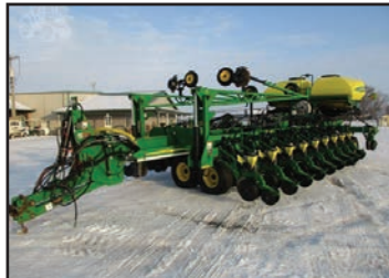
2013 JOHN DEERE DB60 24 Row, 30" Spacing, Precision eSet Meters, Green Star Rate, Active Pneumatic Downforce, Row Command Clutches, Seedstar XP Monitoring-No Display Screen, 2" Banjo Plumbing, Markers, Seed Firmers, Vac, Bulk Fill, (One Owner) $130,000
