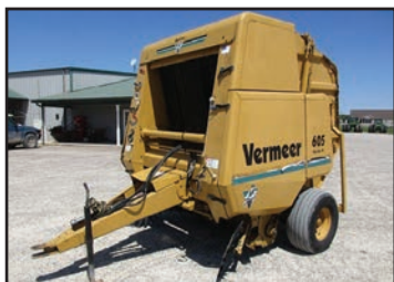
1994 VERMEER 605K 5x6 Bale Size, Twine Tie, Rear Bale Kicker, 540 Pto, Front Kicker Wheels $3,750
