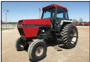
1986 Case IH 2096 5,995 Hours, Power Shift, Small 1000 Pto Interchangeable To 540 Pto, 2 Hyd, Top Link, 5.9 Cummings Engine, 480/80R38 Rear Tires (Note: Tractor Has Clutch Problems) Featured $15,500
