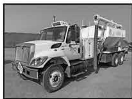
JQ9660 '09 Int'l 7500 ANFO bulk handling truck
