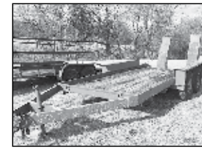
Ditch Witch pull type trailer, stand up ramps
