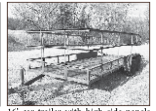
16' car trailer with high side panels for tile pipe
