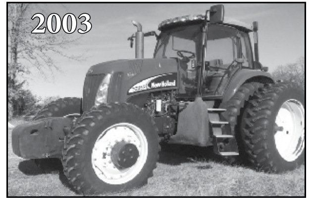
2003 New Holland TG255 4WD cab tractor, 255hp turbo charge diesel engine, power shift, 1000 PTO, 4 hyd outlets, buddy seat, 14.9-34 front tires, 18.4-46 rear tires, duals, good tires, 2 sets inner rear weights, set of 9 front weights, reads 144 hours on replaced tach. Seller believes tractor to have 4000 plus total hours.
