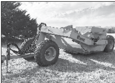
Toreq 13000 by Steiger 13yd. dirt scraper, hyd. eject, front dolly wheels, 16.9-24 tires
