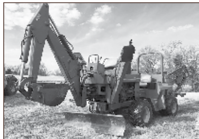
Ditch Witch 6510 trencher, backhoe, 18in bucket, 6ft backfill blade, diesel engine, reads 2143 hours
