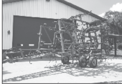
Sunflower 5034-25 ft field cultivator, walking tandems, 9 inch sweeps, 5 bar harrow, Ser 5099-193
