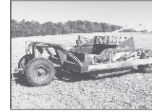
Soil Mover 75R1 pull type scraper, Ser 1D1 6038
