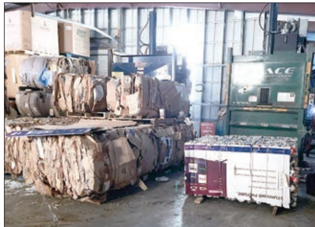
A baler for cardboard on the left and one for plastic on the right.
