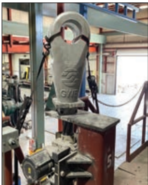
George Washington Bridge socket leveled and centered on wire rope, ready to be poured.
