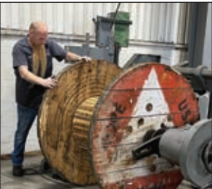
Worker setting up reel to package final wire rope assembly.
