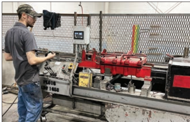
Worker performs non-destructive test to ensure end termination is secured to wire rope.
