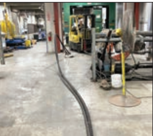
The rope is stretched across the factory floor to work out any imperfections.
