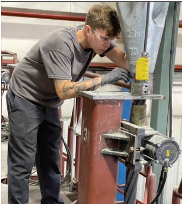
A worker attaches the end termination socket to the rope.
