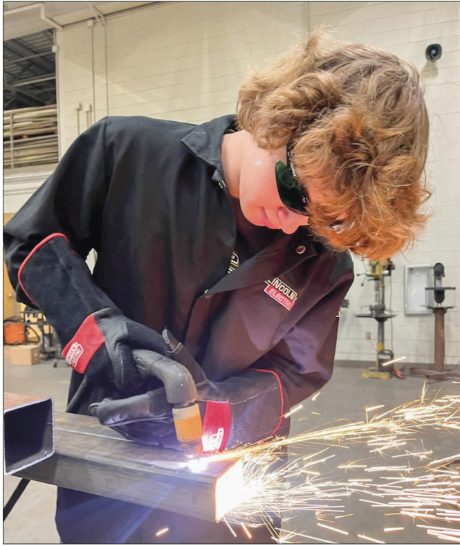
Bryson Wann operates a plasma cutter in a Granbury ISD welding/metal fabrication class, which is part of the agricultural mechanics program.
