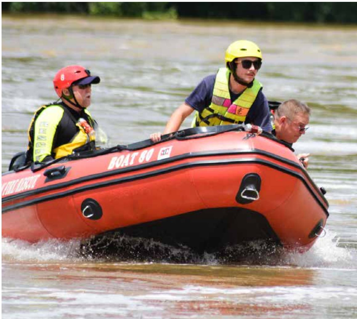
This Inmar inflatable boat with a 40-horsepower outboard engine is used in swift water rescues. It can carry a trained driver and two spotters/divers who can enter the water for rescues.
