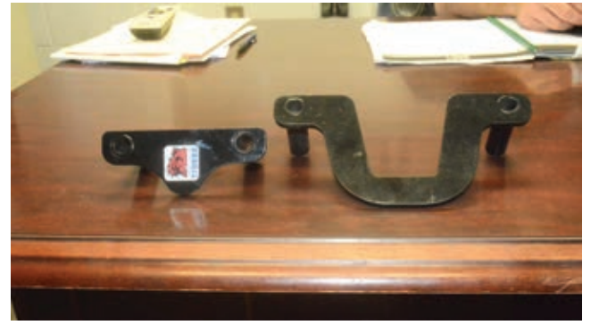
This Z-Lock is for doors that swing in. The particular school's insignia sticker is always on the lock. When a teacher gets flustered, he or she can remember that the sticker side of the lock is always "up."
