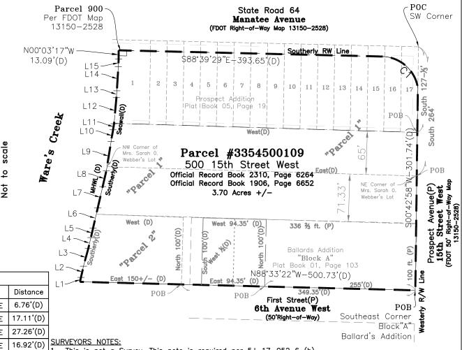
Line Table Bearing Line# N12°39'31"E L1 L2 N12°46'37"E L3 N15'10'26"E L4 N13°20'37"E L5 14.16'(D) N13'07'25"E 30.96'(D) 16 N12°59'36"E L7 N13°04'44"E 32.90'(D) 18 N13°00'53"E 24.46'(D) 43.76'(D) L9 N09'11'57"E L10 N09°29'30"E 17.87'(D) 9.20'(D) L11 N09°21'12"E 38.95'(D) L12 N05'12'39"E L13 N03°38'41"E 10.26'(D) 36.01'(D) L14 N03°24'49"E
