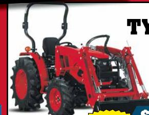
25HP, 4WD, W/LOADER, 2200 LB LOADER LIFT CAPACITY, 12X12 SHUTTLE SHIFT TRANS, 3022 LBS TRACTOR WEIGHT ONLY
