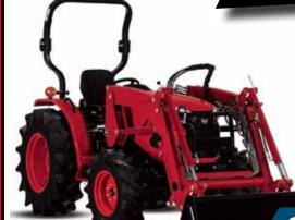
25HP, 4WD, W/LOADER, HYDROSTAT TRANS, 1,378 LBS LOADER LIFT **CAPACITY**
