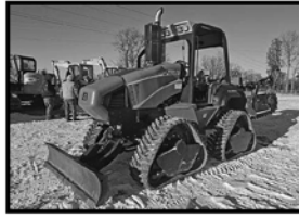
NP9325 '12 Ditch Witch RT115 trencher
