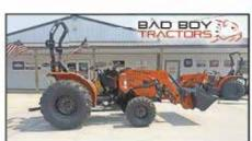
Bad Boy 4035H Tractor, HST, Loader, 4wd, 35hp, industrial tire, 2200lbs loader lift capacity
