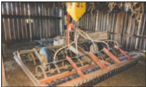
(Figure 1) Seeding clover does not have to be the same old thing. This old cultimulcher frame was modified by adding an air seeder that will handle clover seed. The combination of light harrowing, good seed placement and rolling with the rear rollers is an innovative way to increase the chances of success with clover.
